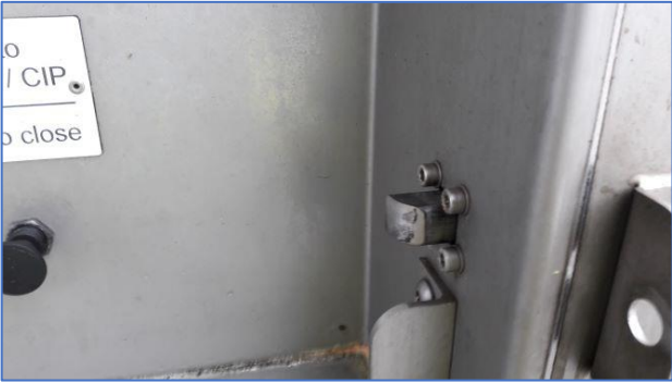
Rear cabinet locking point deployed
